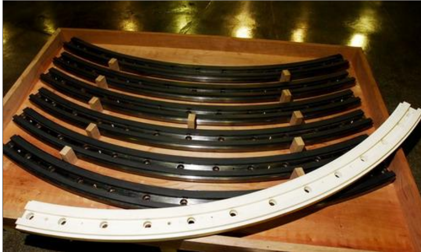
An assembly of a completely recovered gasket and the elastomer (white): two achievements of Itaipu.
