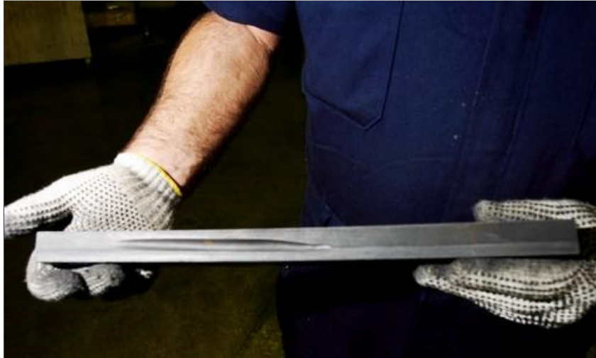
A technician shows the eroded carbon segment: the wear is a common problem regarding the old material.
