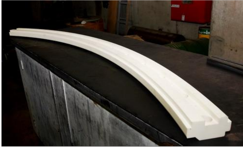
Elastomer gasket segment: the innovative material has been evaluated for three years and has been approved.
