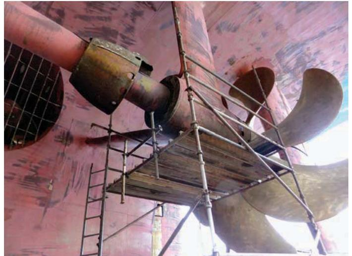
**The port strut of *Grand Princess* with rope guard intact for easy bearing access**
