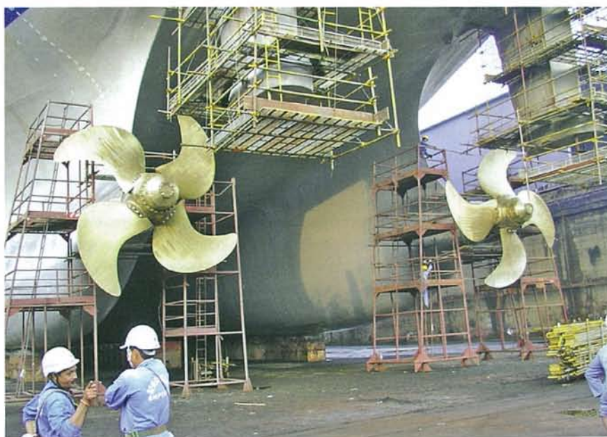
A 142,000dwt tanker equipped with seawater lubricated propeller shaft bearings.
