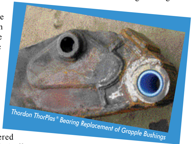
Thordon ThorPlas® Bearings Installed on Berman Brothers Grapple
