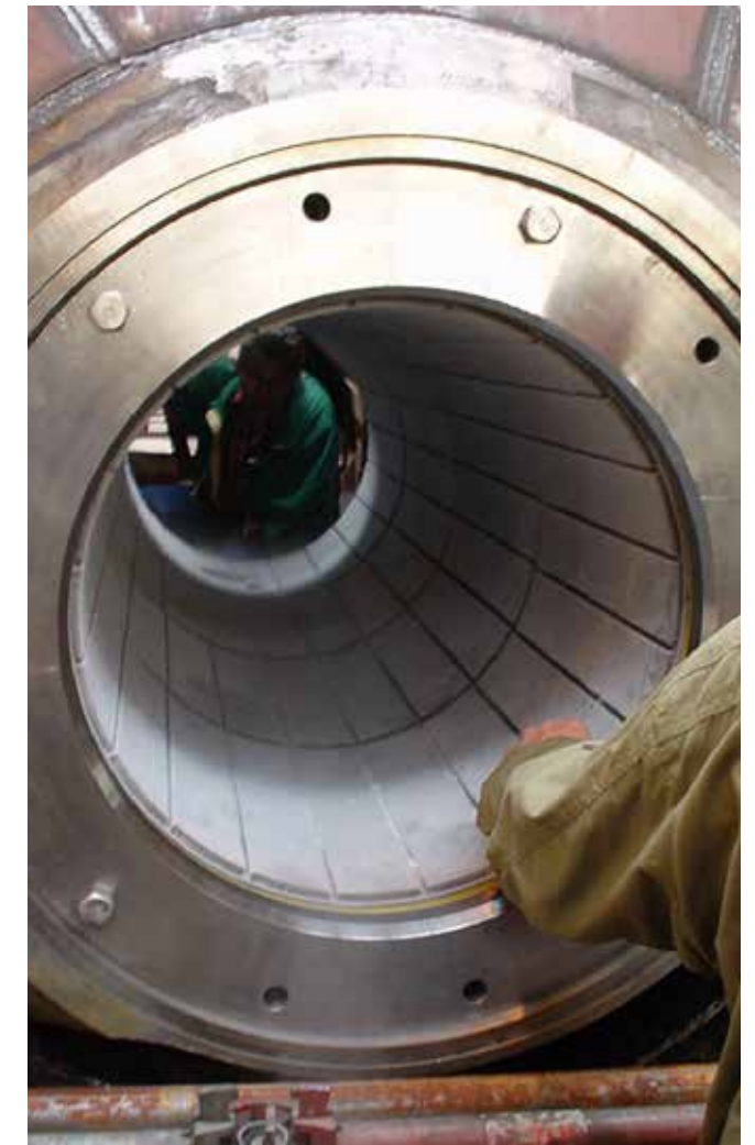
Composite Cutterhead Shaft Bearing installed 2007 to the Royal IHC-built dredger Al Mirfa
