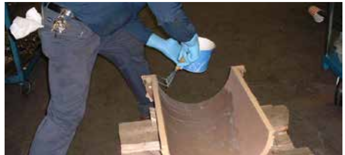
Figure 39: Adhesive being applied to split metal housing
