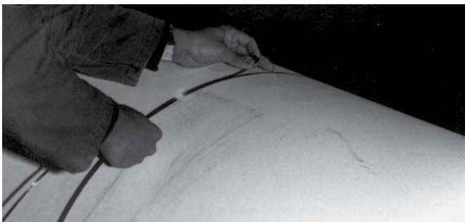
A pi tape is a precision steel tape calibrated to measure diameters by measuring circumference.
