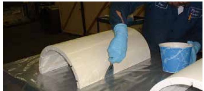
Figure 40: TG-75 being applied to OD of split SXL bearing
