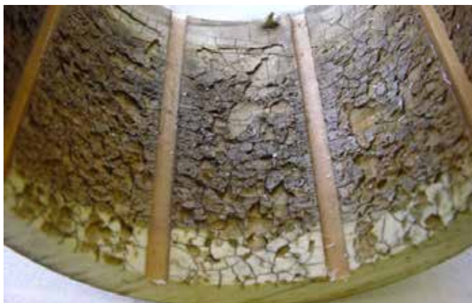
Typical example of bearing with hydrolysis.
