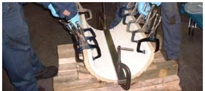
Figure 41: Clamping with slight force SXL to metal housing
