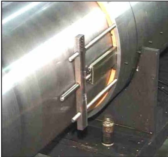
Figure 4. Single Key removal using key extraction tool
