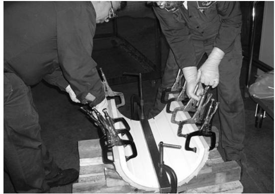
Figure 7: Clamping SXL, with slight force, to metal housing.
