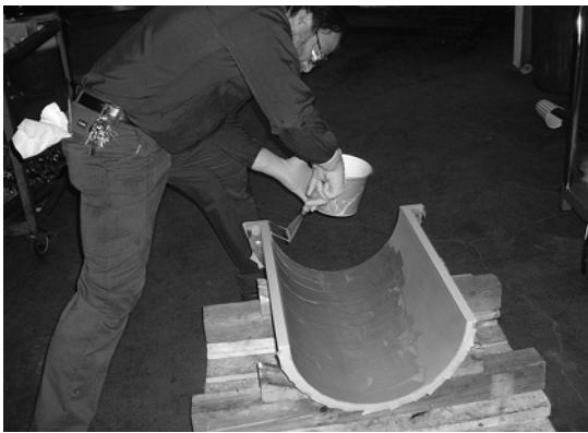
Figure 5: Adhesive applied to split metal housing.
