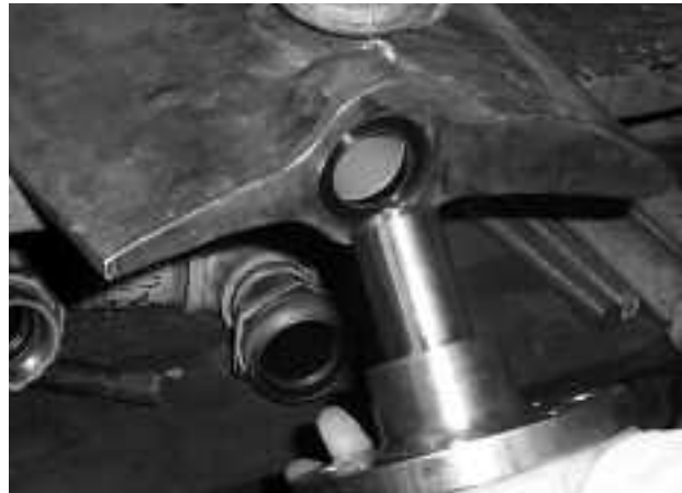
ThorPlas wicket gate bearing with Thorseal
