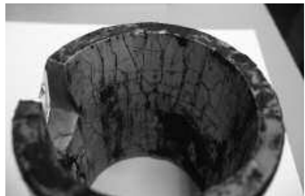
Typical example of ThorPlas bearing with hydrolysis
