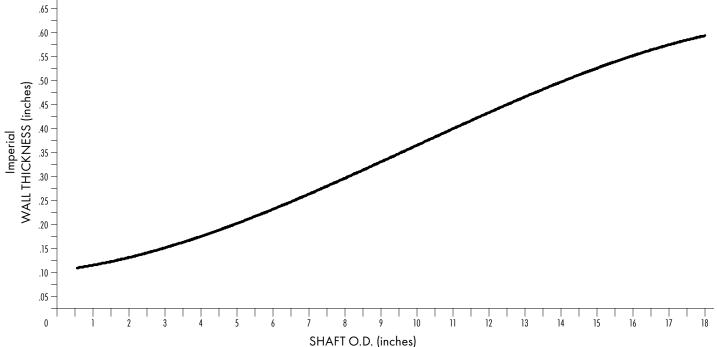
Figure 8: Typical ThorPlas Minimum Wall Thickness Guide
