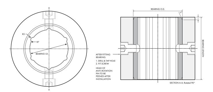
Figure 13: Bearing Retention with Anti-Rotation Pins
