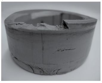
This photograph indicates that the ThorPlas bearing chamfers were too long and as the bearing was loaded in this area, not enough support was available for the material to take the load. Although the bearing cracked, it did not shatter and remained in one piece.
