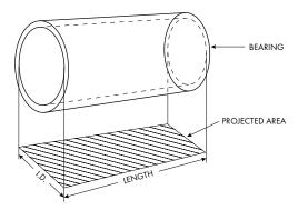
Figure 4: Bearing Pressure
