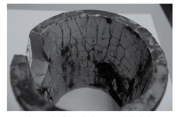
Typical example of ThorPlas bearing with hydrolysis.
