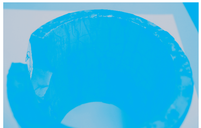
Typical example of ThorPlas bearing with hydrolysis.
