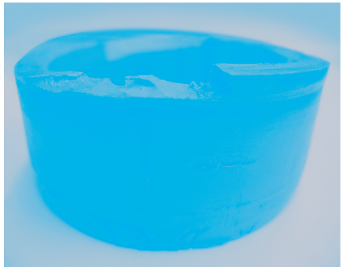
This photograph indicates that the ThorPlas bearing chamfers were too long and as the bearing was loaded in this area, not enough support was available for the material to take the load. Although the bearing cracked, it did not shatter and remained in one piece.
