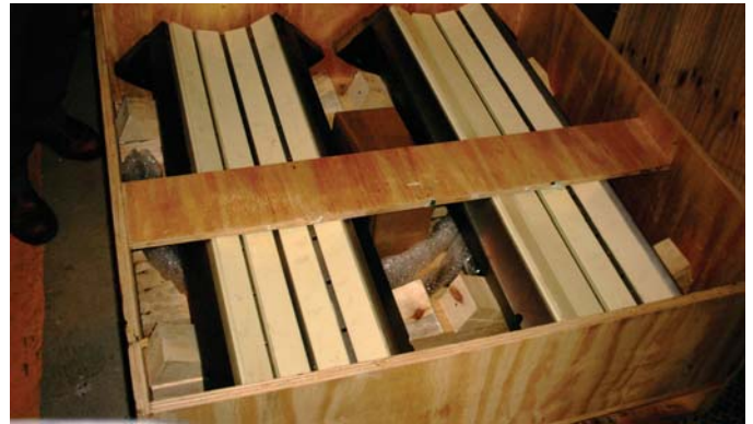
Split SXL Stave Main Guide Bearing
