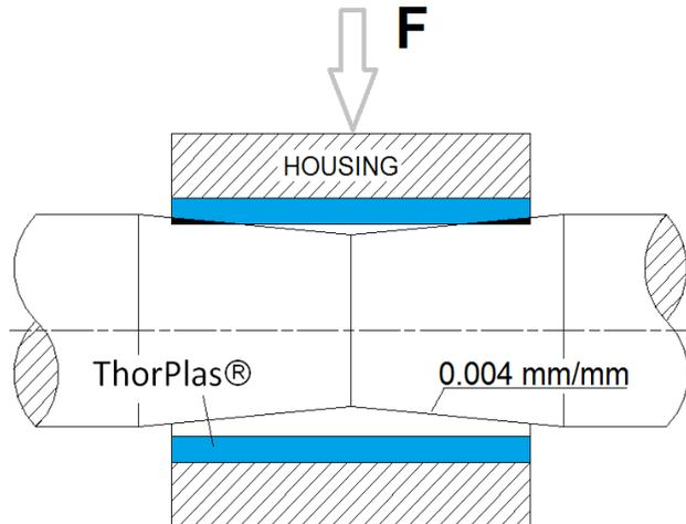
**Fig -9: Friction and wear under edge loading**
