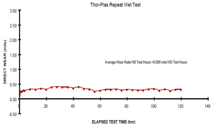
In Fig -2b, after making the initial displacement zero, the calculated wear rate for wet test was actually lower than dry condition. The average adhesive wear during 100 hours was 0.08 mils (1 mil = 0.001 inch)
