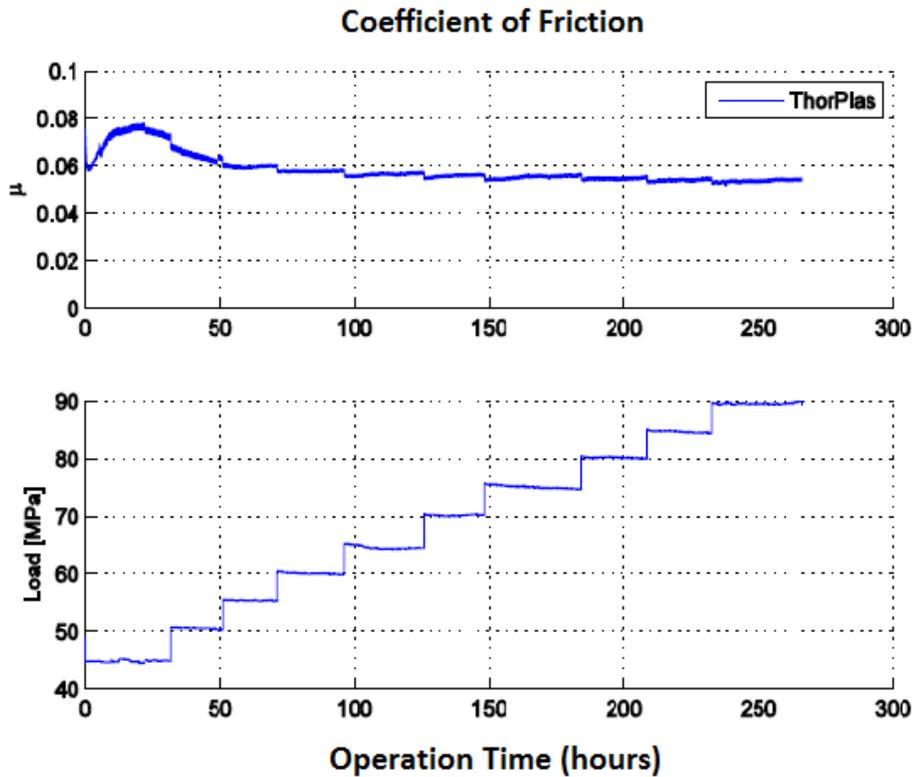
The bearing wear and operational cycles were measured for each pressure level. The result is summarized in Table -1. Based on adhesive wear measurement of the same test, a wear factor can be calculated. The wear factor is defined based on the wear law in common practice:
