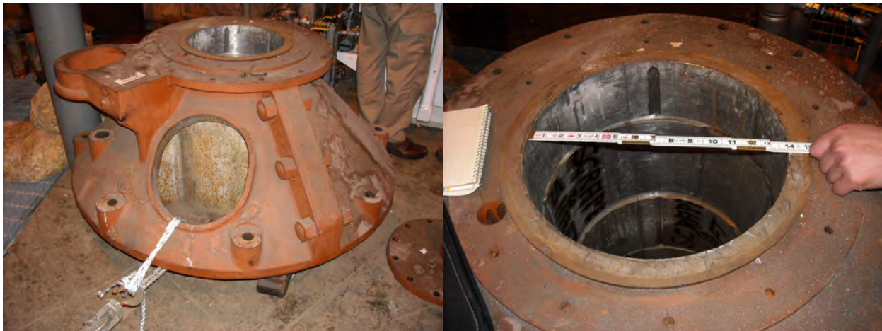
Figure 1: Original Spare White Metal Bearing & Carrier.
