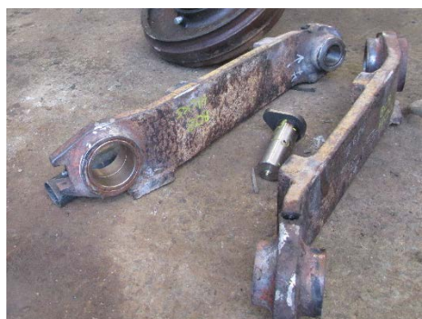
Elevator Support and existing Steel Bearings
