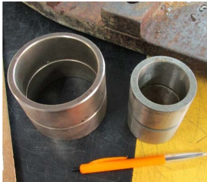
Old Steel Bearings
