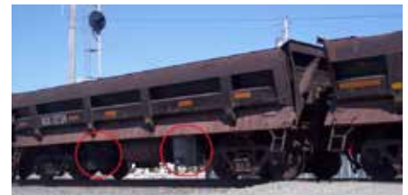
Pneumatic cylinders installed on the mining dump wagons
