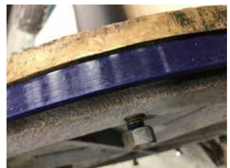
A close-up view of the Thordon Thor-Flex seals installed in a refurbished pneumatic cylinder
