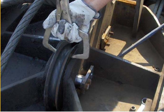
Kronos roll-off truck pulley system used in roll-off trucks
