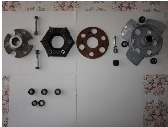
MUTC disassembled trolley bus hardy clutch system
