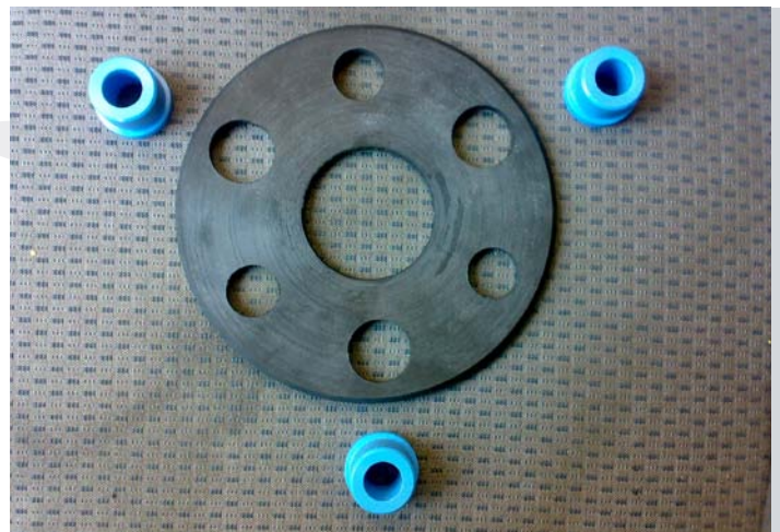
Replacement of clutch Tecamid parts with ThorPlas-Blue
