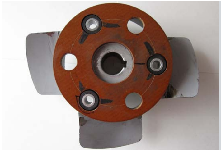
Replacement of clutch Pentinax part with Thordon XL
