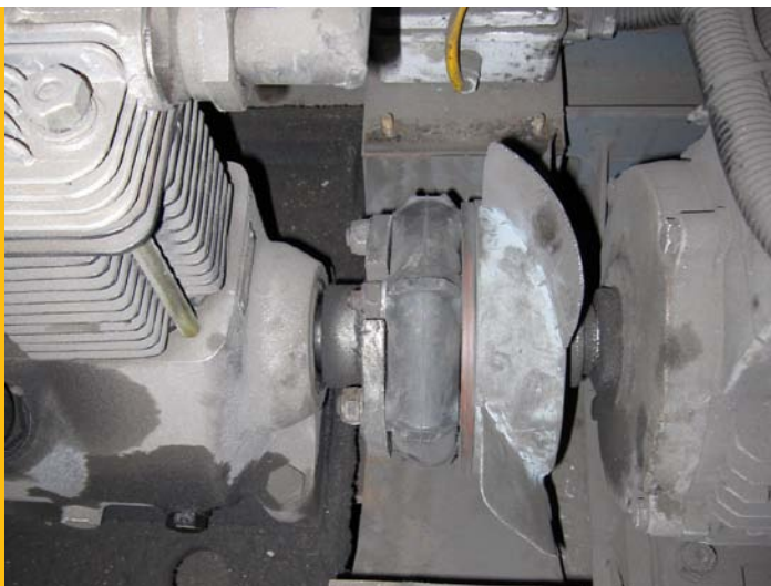
MUTC public trolley bus hardy clutch system
