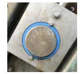
In 2018, Fleetwood Industrial Products, received the order to bore out the housings, install ThorPlas-Blue and refurbish the mating hardware.
