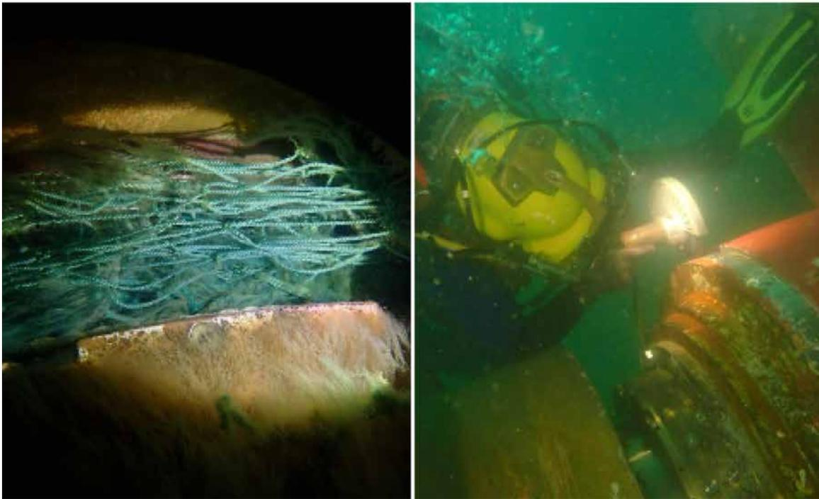
Recently one of our diver/technician teams carried out a double underwater stern tube seal repair on a RORO ship berthed in Port of Burnie, Tasmania. The ship was suffering from an oil leak, making an on-site repair necessary. Using two Hydrex flexible mobdocks simultaneously the team was able to carry out the entire operation on-site and underwater, saving the owner an expensive and time-consuming trip to drydock.
