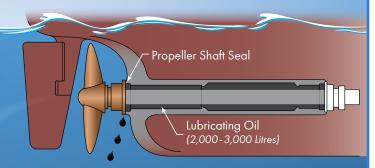
Oil emissions from commercial shipping propulsion systems is a serious problem and can be eliminated with the use of open seawater lubricated propeller shaft systems.
