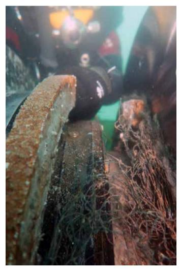
Next the split ring was removed and brought to the surface to be cleaned. The divers then removed the first seal and replaced it with a new one which was bonded. Next, they did the same for the other two seals.
