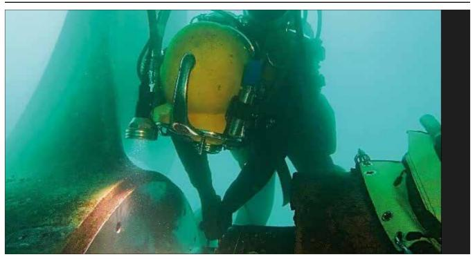
Recently, Hydrex diver/technician teams were deployed to ships in Belgium and Spain for stern tube seal replacements. The first operation took place in Algeciras on a 225-meter container ship, while the second was carried out in Antwerp on a 295-meter RoRo vessel.
