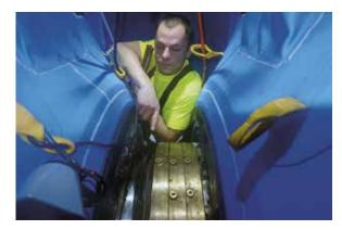
Double Stern Tube Seal Repair on RORO Vessel in Tasmania
