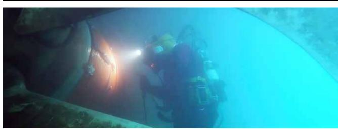
Earlier this year our diver/technician teams carried out a double underwater stern tube seal repair on a RORO ship berthed in Port of Burnie, Tasmania. The ship was leaking oil, making an on-site repair necessary. Using two Hydrex flexible mobdocks simultaneously the team was able to carry out the entire operation on-site and underwater, saving the owner an expensive and time-consuming trip to drydock.
