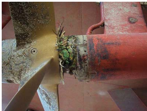
Figure 2: Rope tangled around propeller shaft causing seal damage
