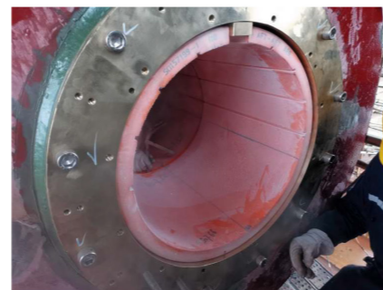
COMPAC Open Seawater-Lubricated Propeller Shaft Bearing System (above).
