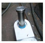
The ThorPlas-Blue SAB and hard coating pin system can be ordered in 4 standard pin sizes: 1.5", 2", 2.5", and 3", as well as in custom sizes.
