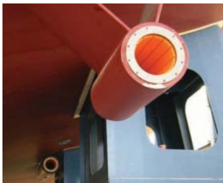
Thordon COMPAC Starboard Strut Bearing Installed on Mega Yacht
