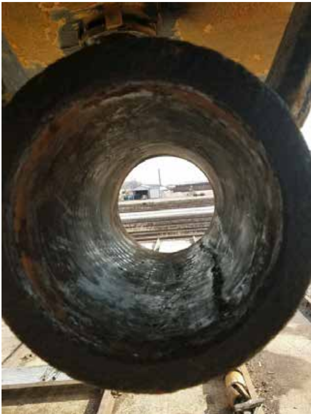
Strut tube before machining and after with RiverTough bearing installed.
