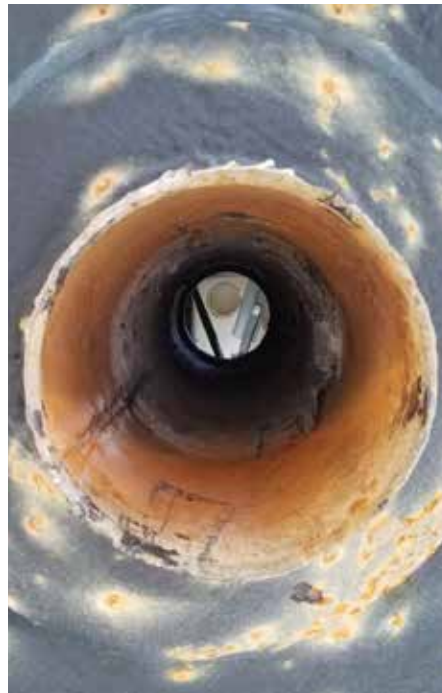
Rudder housings bored and SXL bearings installed.
