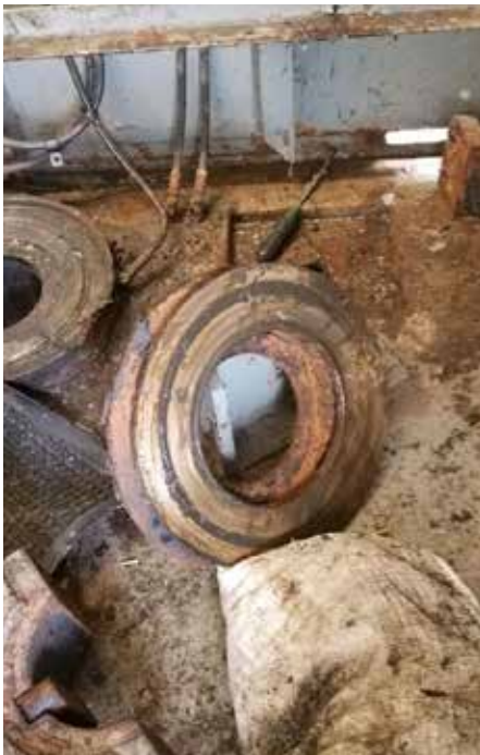
Rudder housings bored and SXL bearings installed.
