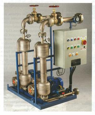
the water stream, then collects it and discharges it through a blow down line." The new approach features its own pumps, separators and flow monitoring equipment.
