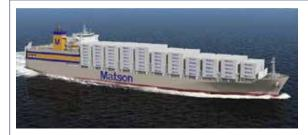
Matson Navigation Co. Inc. (USA) 2 – 51,400 DWT 3600 TEU container ships Equipped with COMPAC system, WQP & ThorShield Delivered: 2018 - 2019 Philadelphia Shipyard (USA)
