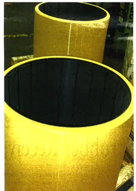
Thordon Composite cutterhead shaft bearings prior to installation on the D'Artagnan owned by DEME
