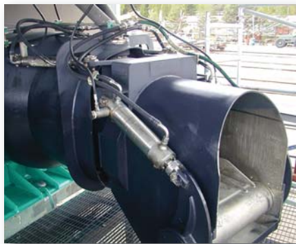
Water jet nozzle equipped with water lubricated Thordon GM2401 line bearings
