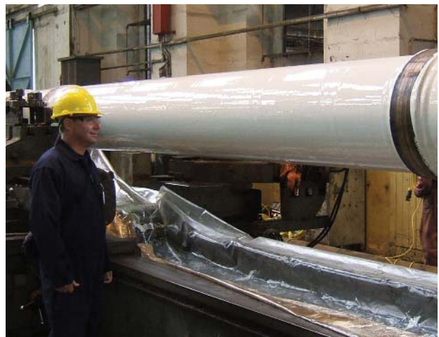
Thor-Coat propeller shaft coating for 563.5 mm (22.185") shafts of Marco Polo cruise ship
