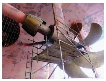
The port strut of *Grand Princess* with rope guard intact for easy bearing access
