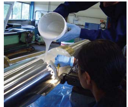
Easily applying one coat Thor-Coat using a doctor blade mounted on a lathe
