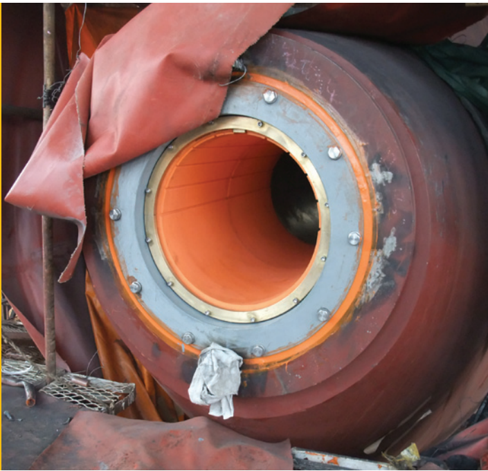
Installation of Thordon COMPAC seawater lubricated propeller shaft bearing on CSL bulk carrier built in China
