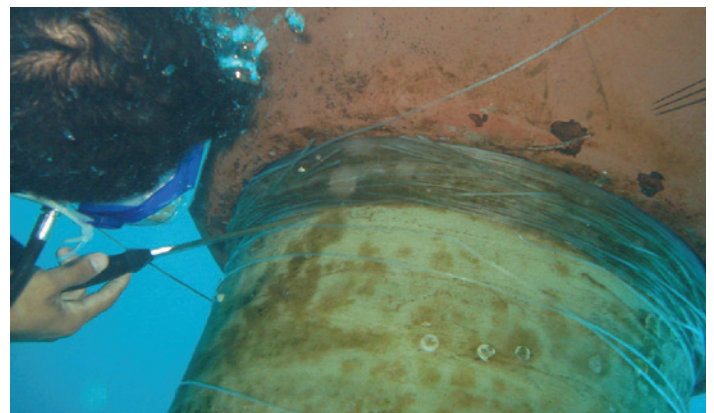
Aft shaft seal damage caused by fishing net caught in the propeller
