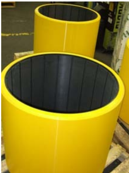
Thordon Composite cutterhead shaft bearings prior to installation on the D'Artagnan owned by DEME
