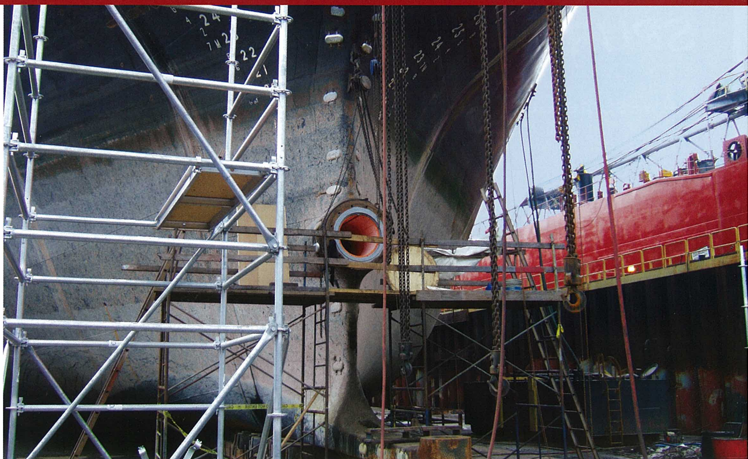
Thordon Compac bearings in the sterntube of the bulker Peter R Cresswell
