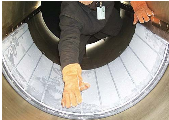
Easy installation of split XL propeller shaft bearings with tapered double key design allows bearings to be removed without shaft withdrawal
