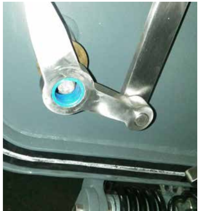
Closing device with ThorPlas-Blue bearing installed
