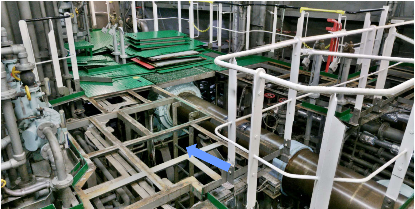
Prototype vessel's sterntube lubricating oil drain tank (5.2m 3 )
