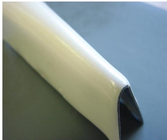
FIGURE 5 Conical Mandrel Bend Test (Thordon Bearings R&D Laboratory, ON, Canada, 2004)
