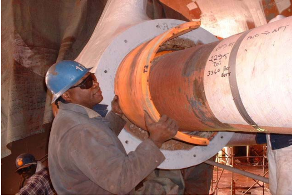
Figure 6: Single tapered keyset allows for easy removal, inspection and re-install in a matter of hours without shaft withdrawal
