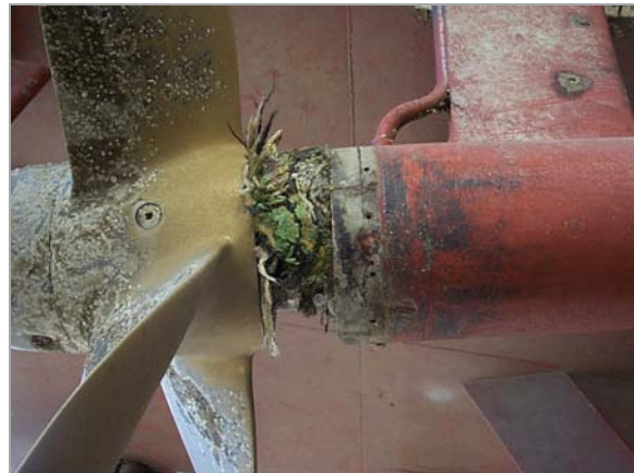
Figure 2: Ropes and fishing line damage aft seals
