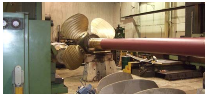
Figure 6. Shaft coated with a tin-free anti-fouling paint.
