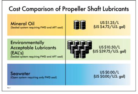
The intention of this White Paper is not only to raise awareness of the commercial disadvantages and environmental damage created from the continued use of oil lubricated propeller shaft bearing systems, but also to offer a more cost-effective and more environmentally acceptable solution:
