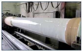
A key difference between the oil and seawater lubricated system is that the latter technology requires a means to protect the propeller shaft against seawater corrosion. Fortunately, shaft coating technologies have significantly improved since the early days of water lubricated bearings. And today, two-part polymer coatings have been developed to keep the propeller shaft corrosion free. Typically, bronze liners, Inconel™ or welded cladding are used in way of the bearings.
