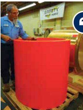
*“We chose the propeller shaft bearings for this vessel because these bearings are environmentally friendly, water lubricated and come with no risk of pollution.”*
