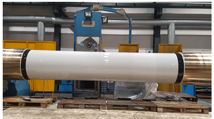
Fig. 6. New 2-part epoxy corrosion resistant propeller shaft coating
