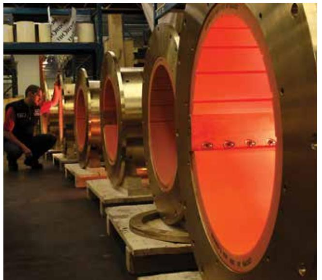
*Viking Jupiter*, the 47,800gt cruise ship built at Fincantieri's shipyard in Ancona, Italy for Viking Cruises, has been delivered with a Thordon Bearings' seawater-lubricated propeller shaft system. It is the sixth Viking cruise ship to be fitted out with the COMPAC bearing arrangement.
