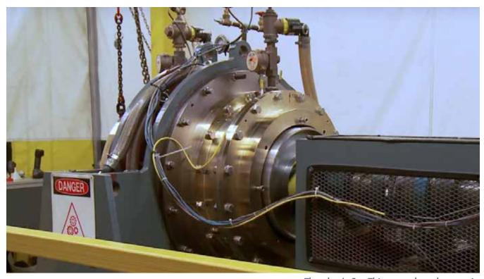
Thordon's SeaThigor seal on the test rig
