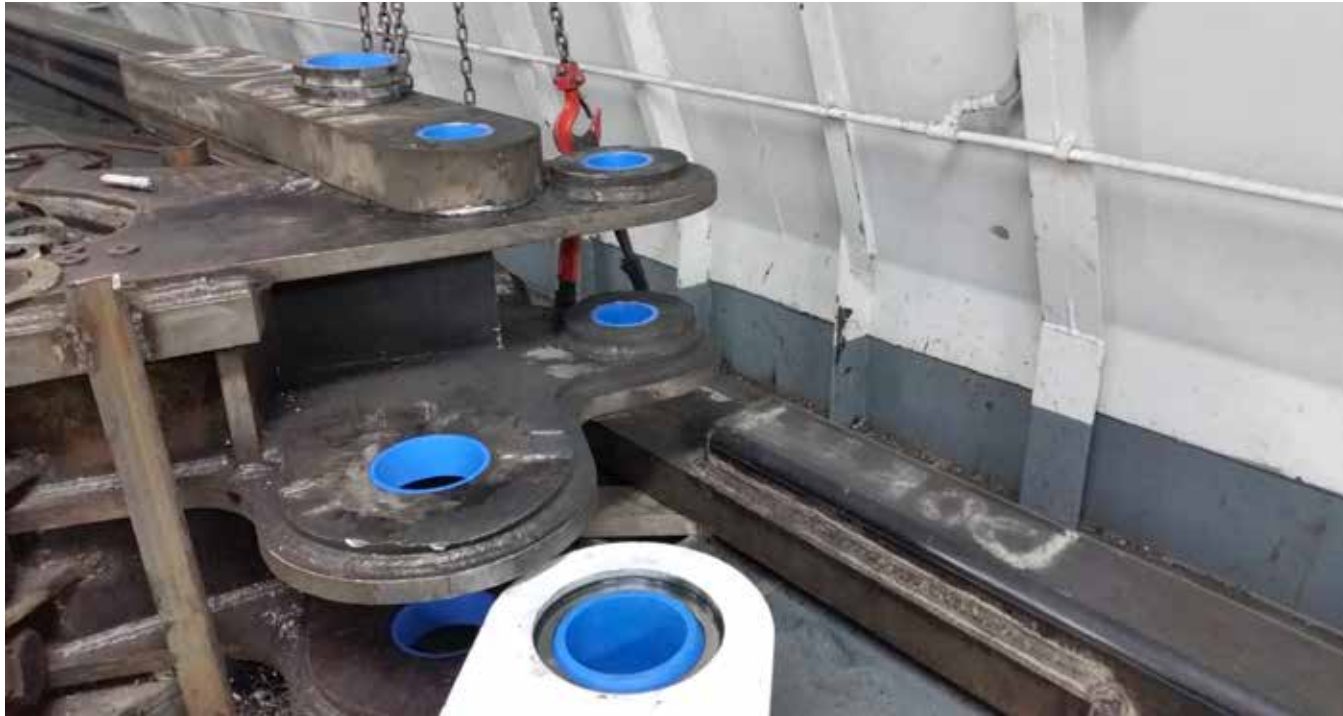
ThorPlas-Blue installed in tiller arm application
