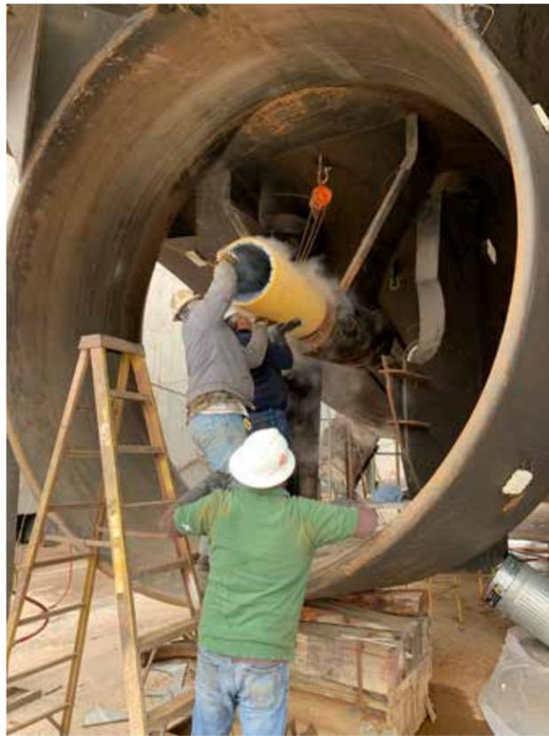
During a recent drydocking, the final vessel in a series of five ship-assist tugs was successfully converted to RiverTough tailshaft bearings and Thordon's TG100 shaft seals and returned to work on the Mississippi River.
