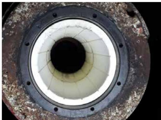
The 1903-built steamship, rescued from scrap merchants 15 years ago, was fully restored in 2016 at Birkenhead's Cammell Laird yard, the original builder of the vessel. Thordon Bearings' SXL water lubricated propeller shaft bearings were installed last year after competitor bearings failed.
